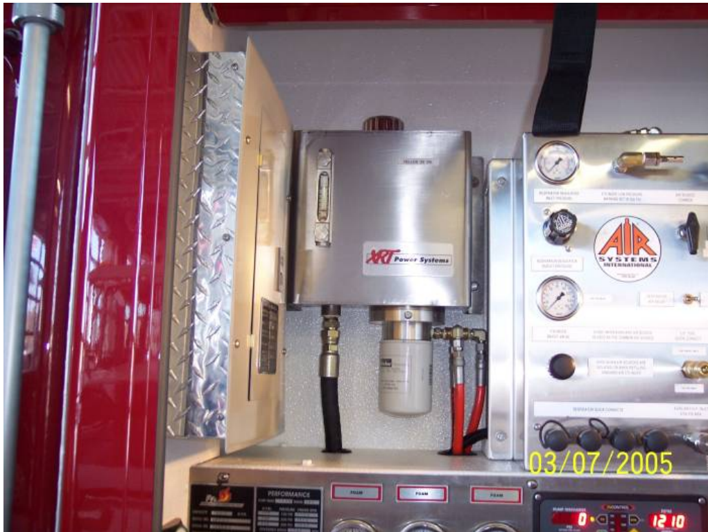
Photo 10 Remote oil reservoir tank w/filter mounted
